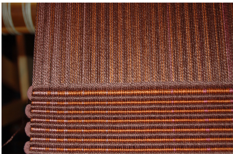
Fig 3: Open shed. Using the weft to the left of the pulled-up loop, pull out slack at left selvedge. Beat weft again.
