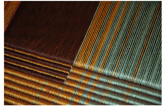
Fig 5: Pull out slack from right selvedge. Beat weft in place
