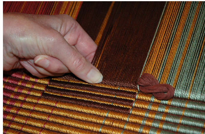
Fig 4: Keep shed open. Insert left index finger into shed. Pinch weft between finger and thumb.
