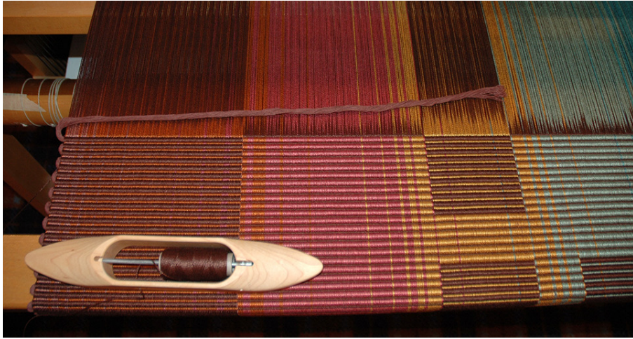
Fig 1: Thick pick is too heavy to overlap when adding new weft. Thick-pick wefts have to be spliced.
