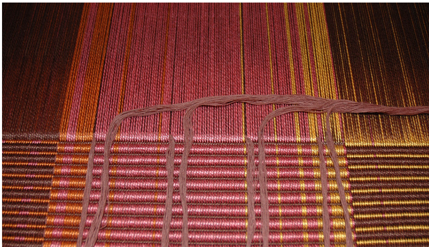
Slit 1 Slit 2 Slit 3 Slit 4 Fig 3: Replacement weft will "back in" from the right side. Open shed. With a 9" tail, pull out the full weight at Slit 4. Divide into four equal-weight tails. Leave 1/4-weight tail in Slit 4. Insert the 3/4-weight tail into shed. Moving towards the left, pull up 1/4-weight tails in Slits 3, 2, and 1.
